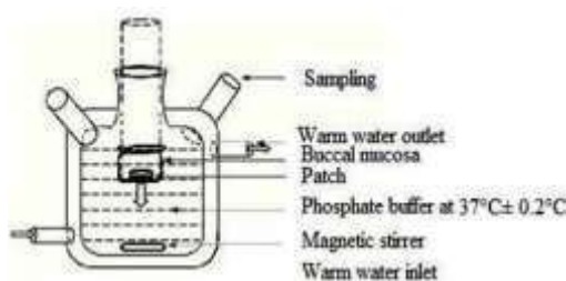
Fig.8: Schematic diagram of Franz diffusion cell for buccal patch
