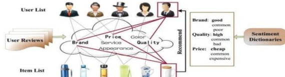
Fig. 1. The product features that user cares about are collected in the cloud including the words "Brand", "Price", and "Quality", etc. By extracting user sentiment words from user reviews, we construct the sentiment dictionaries. And the last user is interested in those product features, so based on the user reviews and the sentiment dictionaries, the last item will be recommended.
